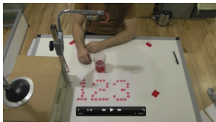
Fig. 2 Robotic display using liquid as medium.
